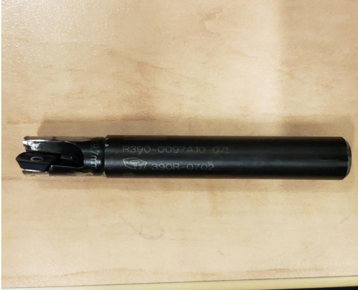
Figure 3.6 Tool holder for the inserts.
